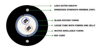
\*Typical Construction Diagram - Not to Scale
